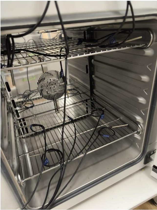
Fig.2. Location of temperature measurement sensors in the climatic chamber's useful volume
