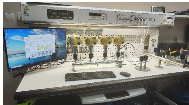
Fig. 1 Automated inspection bench
