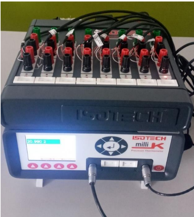
Fig.3. Calibration complex based on the "millik" precision thermometer
