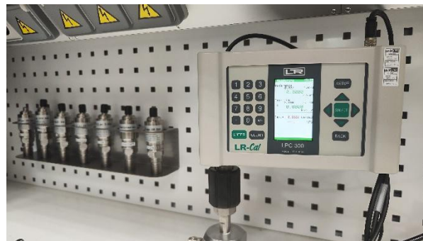
Fig. 2 LR-Cal reference standard electronic pressure calibrator
