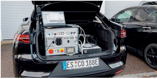
Figure 4 - Mobile measuring laboratory in the trunk
