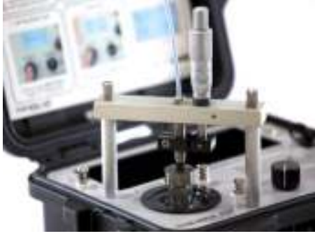
Fig. 2 Vibration stand for verification of the measurement variables of accelerometers and eddy current sensors
