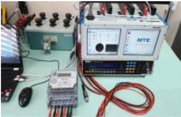
Fig. 3 Check of energy meters
