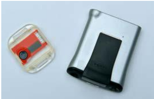
Fig.2. Passive thermo luminescent dosimeter and individual electronic dosimeter.
