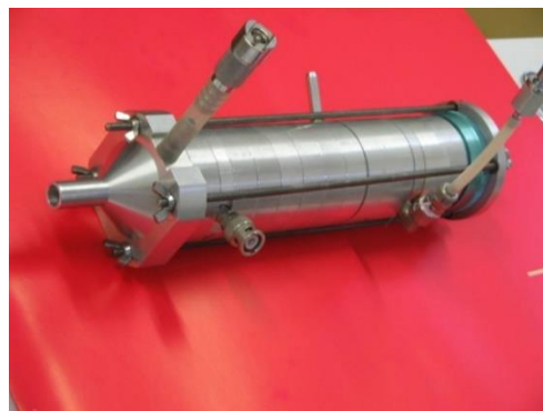
Fig. 8. Aluminum cassette implementing the "double filter" method.
